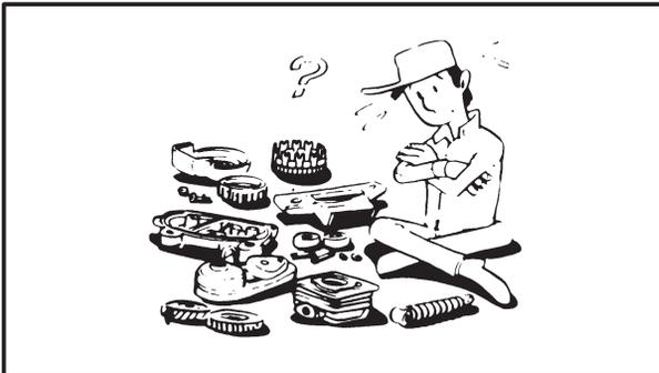
3. When disassembling the machine, keep mated parts together. This includes gears, cylinders, pistons, and other parts that have been "mated" through normal wear. Mated parts must be reused or replaced as an assembly.
